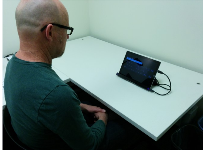
Figure 1. Participants completed 8 sessions of gaze typing tasks using our software. The device shown above is a Microsoft Surface Pro 3 with an SMI REDn eye-tracker mounted at the base.
