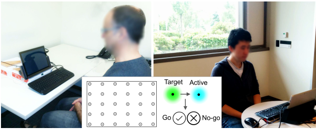
Figure 1. Image of the study setup. Left: in a room with no windows illuminated by artificial light. Right: in a room with large windows facing the tracker, recorded on a cloudy day. Inset: design of targets and go/no-go symbols and their distribution over the screen.
