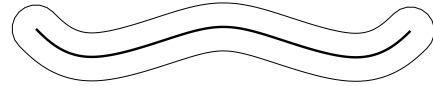
Figure 4: Defining a cross section using offsets and circular end caps — A closed cross section may be defined in terms of a non-closed curve by concatenating two offset curves and two circular end caps.
