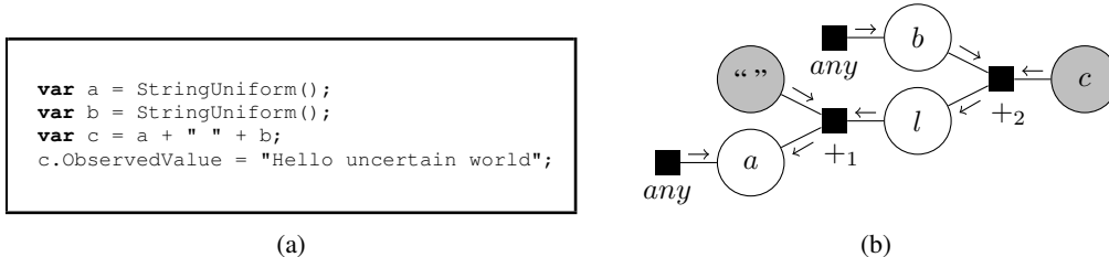
Figure 1: (a) An example Infer.NET program defining a probability distribution over three string variables, one of which is observed. (b) The corresponding factor graph. Subscripts have been added to distinguish between different instances of the concatenation factor. Arrows show the message-passing schedule for computing the marginal of a .
