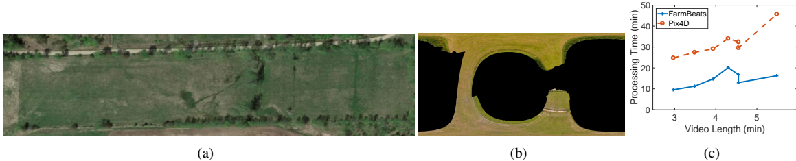
Figure 8: Orthomosaic Generation: (a) The Google Earth image for the farm in Figure 4. (b) Microsoft ICE image stitching pipeline fails to reconstruct it accurately. (c) Pix4D takes about 2.2x longer on average compared to our approach.
