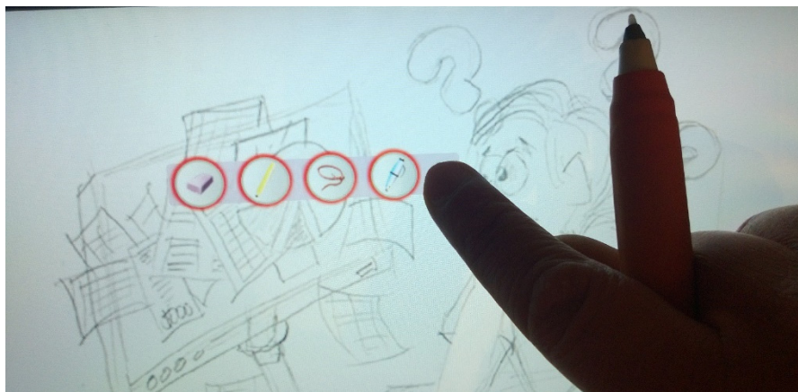
Fig. 10 Tapping the screen with the pen-at-hand brings up the pen tools. Photo © Ken Hinckley, 2014. Used by permission. All rights reserved.
