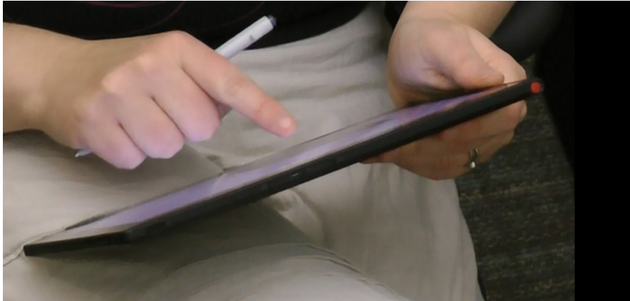
Fig. 4 What input modality is this? At first glance one might dismiss this as a straightforward illustration of a ‘touch’ interaction – a user about to put his index finger to the touchscreen. But a more careful look at the oft seen, but seldom noticed details of how the participant is using the tablet, and the stylus, with both hands suggests that the answer is not so simple. Photo © Ken Hinckley, 2014. Used by permission. All rights reserved.
