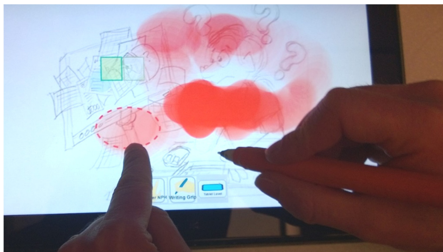
Fig. 12 The airbrush tool. A touch from the nonpreferred hand indicates where to airbrush, while the preferred hand orients the pen in 3D to control the conic section of the resulting spray. Note that the pen does not have to stay “within range” of the traditional ~1cm sensing range of the tablet digitizer during this interaction, because our augmented sensors provide the 3D orientation information. Photo © Ken Hinckley, 2014. Used by permission. All rights reserved.
