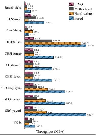
Figure 9. Throughputs for various pipelines
