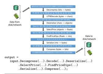
**Figure 1.** Motivating example of a log processing pipeline where an input stream of bits goes through various stages to an output stream of bits. This paper allows programmers to declaratively specify this pipeline as a composition of symbolic transducers, as shown at the bottom.
