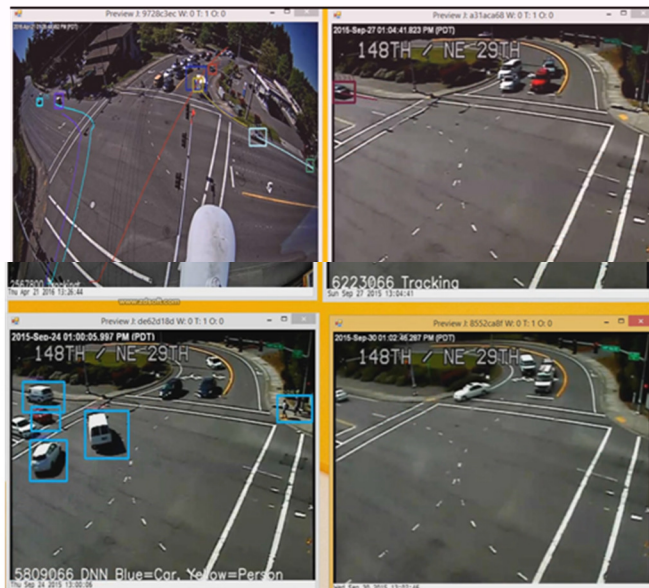
Figure 4: Production deployment details of traffic analytics at Bellevue, WA based on live traffic intersection camera streams. The figure shows a dashboard of multiple camera feeds being analyzed simultaneously, the video analytics pipeline, and temporal graphs of directional volumes.
