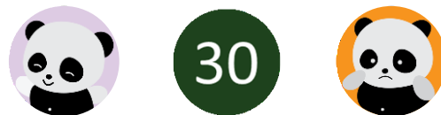
Figure 2. Three possible states of the Plan & Play widget that is displayed in the top right corner above all screen content whenever a plan is active. Widget states: the active app is the planned app (left), counting down before a transition (center), the active app is not the planned app (right).
