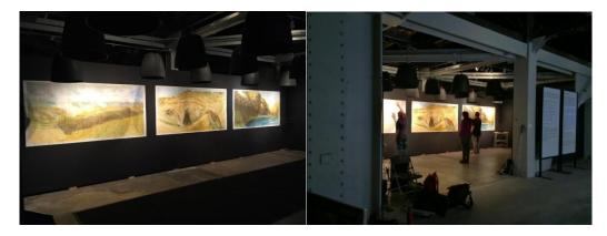
Fig. 5. The Oregon Project on display in October 2016. Three impressionistic drawings are at the front of the room with a four Kinects to track people, and a 3x5 speaker grid overhead. As a person moves and gestures in the space, composed sound tracks that correspond to location relative to the drawings are played overhead. The speaker grid provides a target, individualized sound so that there are both personalized and group experiences occurring in the space.
