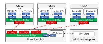
Figure 6: The architecture of management plane. Physical interfaces are omitted for brevity.
