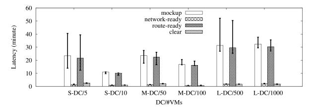
Figure 8: The 10<sup>th</sup>, 50<sup>th</sup> and 90<sup>th</sup> percentile latencies to start/stop emulations with CrystalNet for different datacenter scales.
