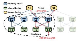
(a) A unsafe static boundary to emulate T1-4 and L1-4.
